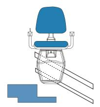
Inclined finished position with optional swivel seat
